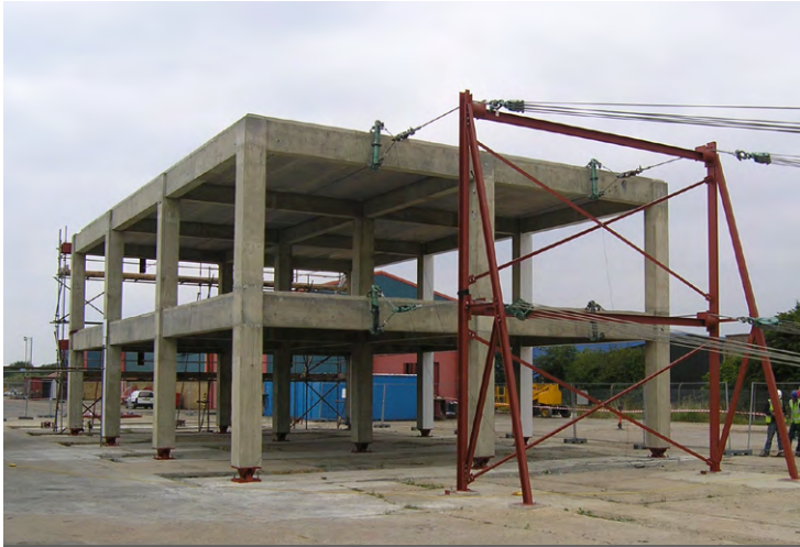
Pull-down tests to validate engineering calculations
